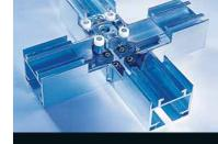
The type R rail system combined with cross-roll carriers is particularly suitable for right-angled branches and intersections. The track rollers mounted in ballbearings exhibit extremely quiet operation and are also maintenance-free. The system is ideal for a very wide range of different layouts and high element weights. Support rollers in the branch junctions and intersections prevent the elements from dropping as they pass through for increased user convenience and easier handling.
