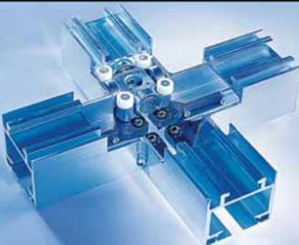
The type R rail system combined with cross-roll carriers is particularly suitable for right-angled branches and intersections. The track rollers mounted in ballbearings exhibit extremely quiet operation and are also maintenance-free. The system is ideal for a very wide range of different layouts and high element weights. Support rollers in the branch junctions and intersections prevent the elements from dropping as they pass through for increased user convenience and easier handling.
