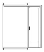
Example of horizontal dimension (width) setting of a structure belonging to a typology made up of two structures
